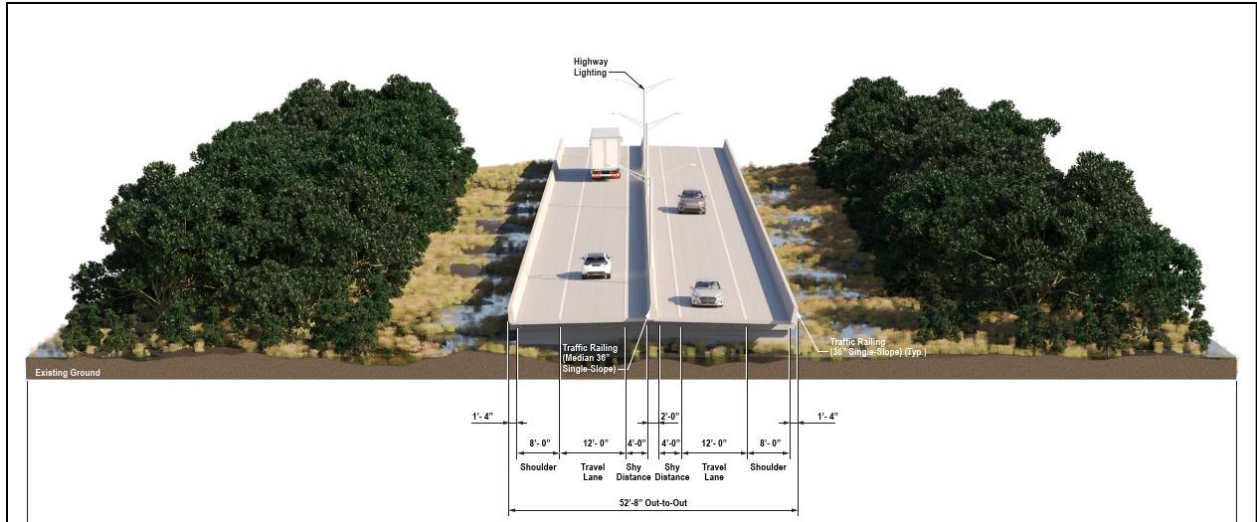
Year 2026 Bridge Typical Section for Alternatives B1, B2, and B3 – Section 2 and Section 3
